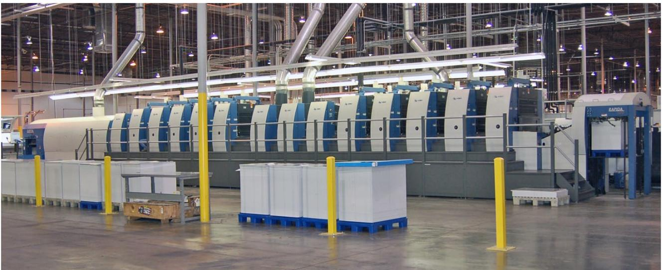
Cartamundi, a major producer of card products and rising commercial packaging printer, installed a new customized KBA Rapida 106 five-over-five 41-inch sheetfed perfector press with full UV capabilities, coating, and board kit at its new facility in Dallas, Texas.
